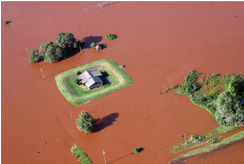
Figure 3-18. A home protected by a levee.
